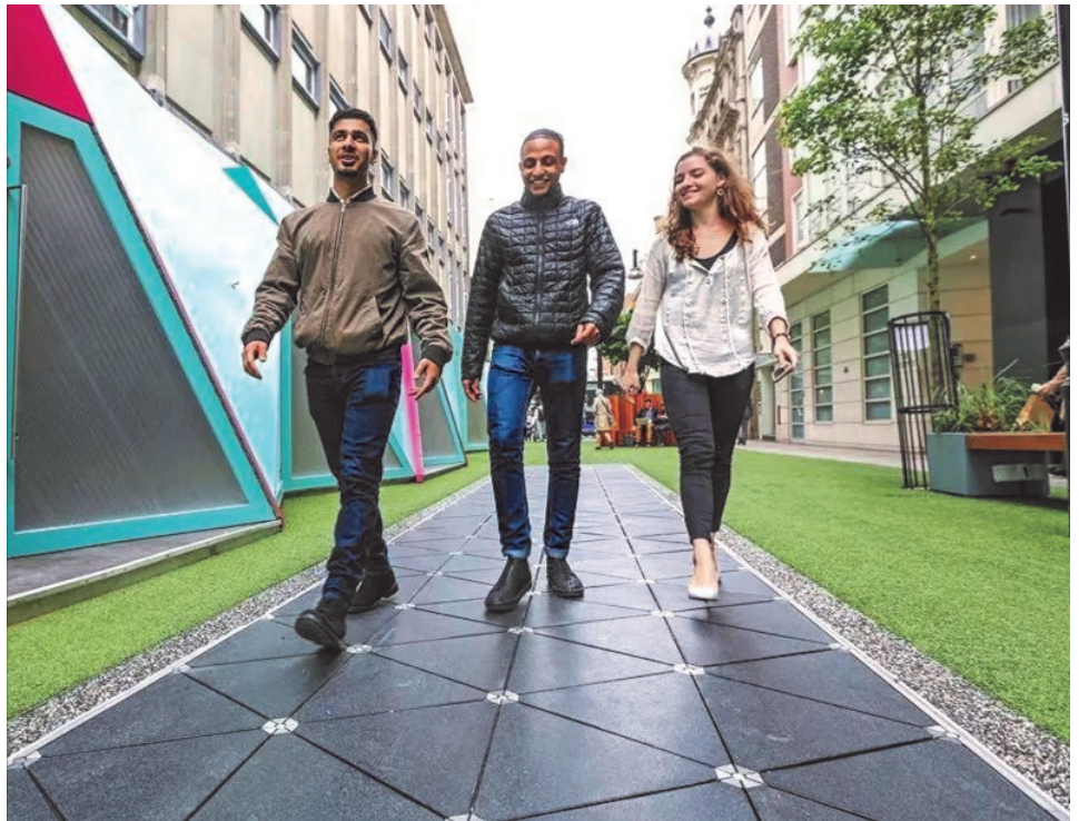
Pavegen pavement which generates electricity from footfall, in Oxford Street.
